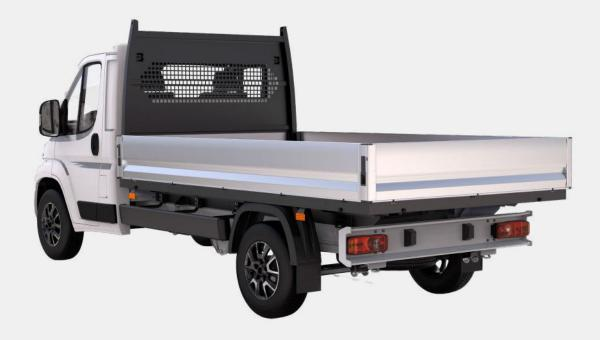
The Ducato dropside features an open platform with fold down side panels to make loading and unloading of goods effortless.
